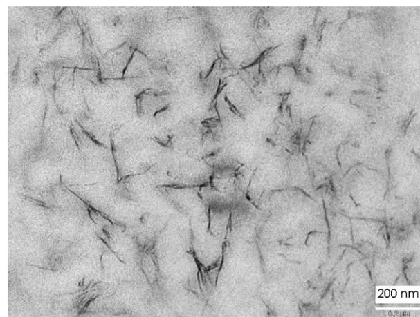
Fig. 4. TEM images of the PHBV/5% CNW nanocomposite film at 75 k magnification.
